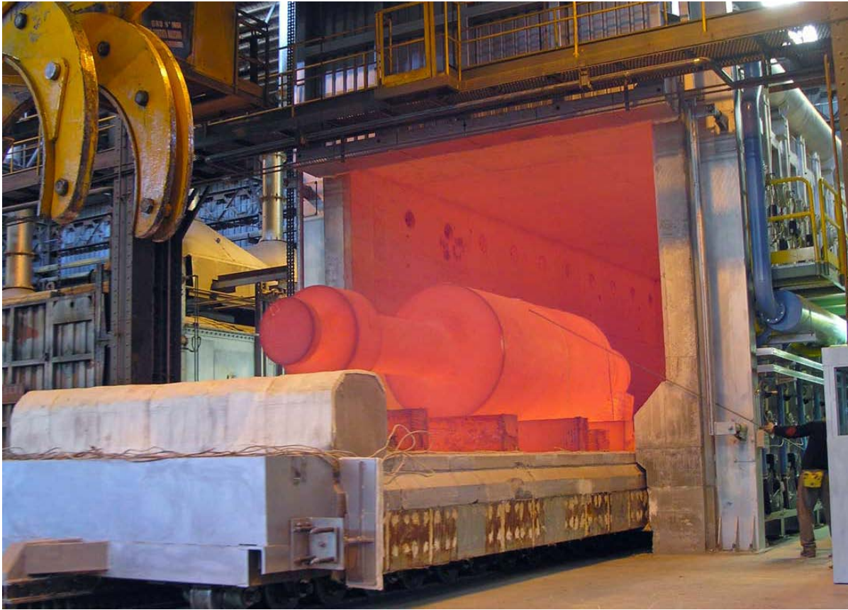
Car Bottom Furnace
